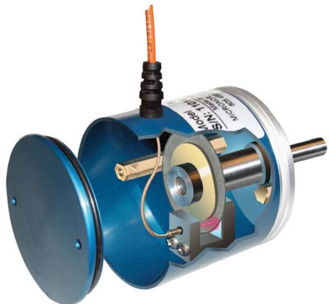
Figure 2. Cutaway view of the Fiber Optic Encoder.
