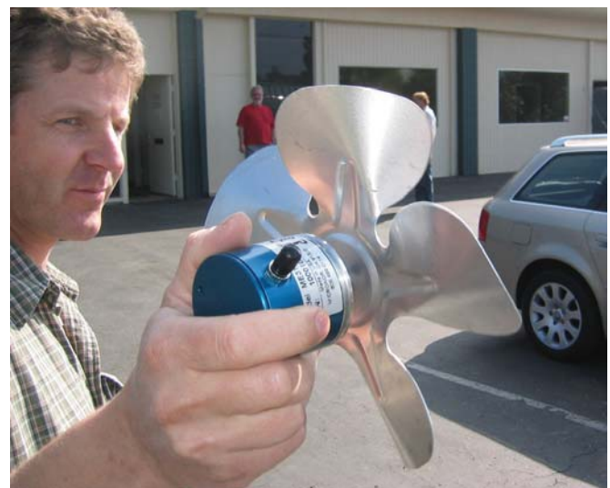
Figure 4. Demonstration of the fiber optic "anemometer" proof-of-concept for measuring air velocity in underground mines.
