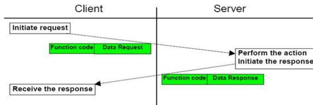
Figure 2: Basic MODBUS Transaction<sup>1</sup>
