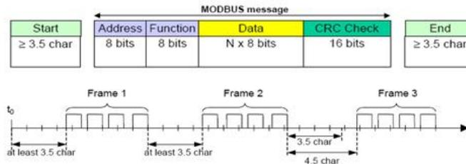
Figure 8: MODBUS RTU Serial Frame<sup>1</sup>
