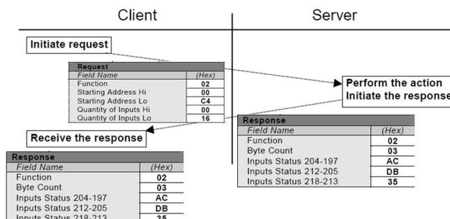
Figure 5: Complete MODBUS Transaction<sup>1</sup>
