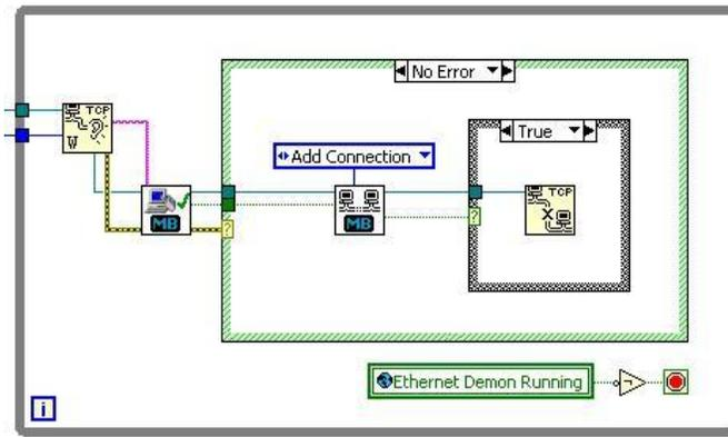
Figure 21: MODBUS TCP Slave Main Loop Part 1
