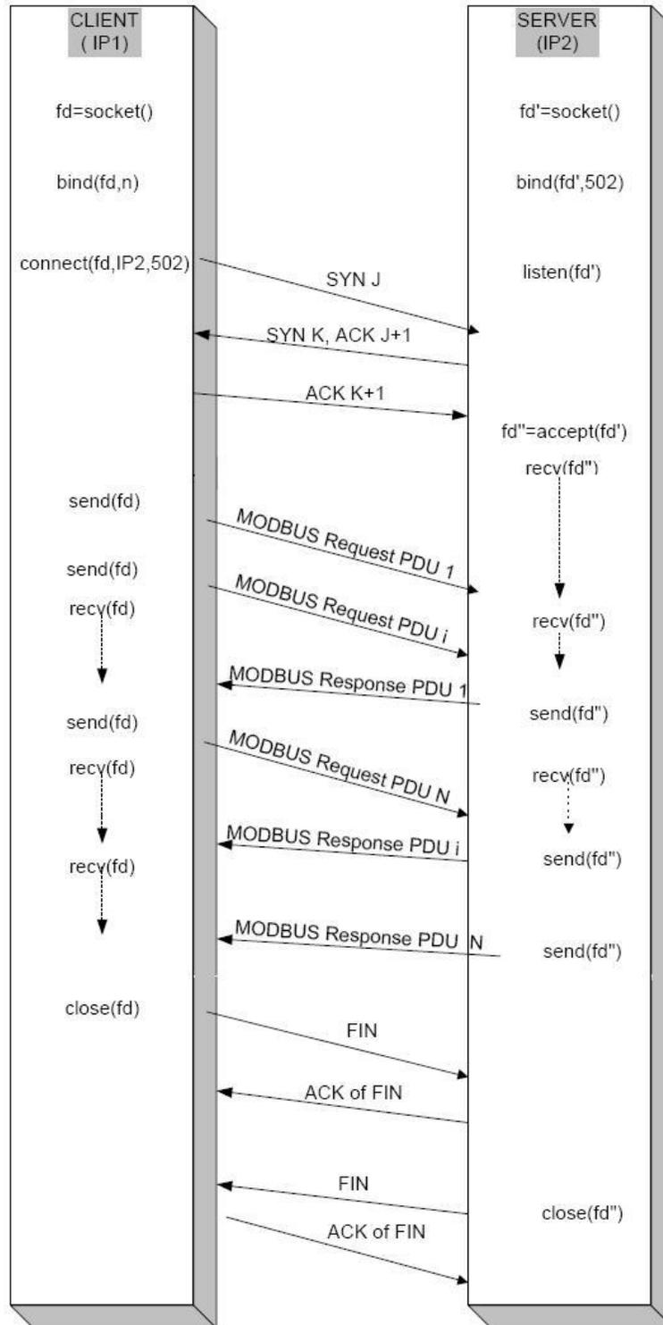
Figure 10: Complete MODBUS TCP Transaction<sup>1</sup>
