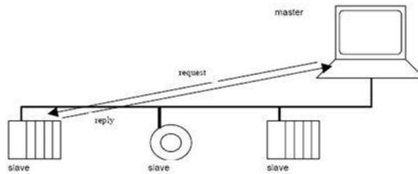
Figure 1: Basic MODBUS Network<sup>1</sup>
