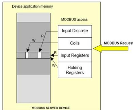
Figure 4: MODBUS Transaction with Data Types<sup>1</sup>
