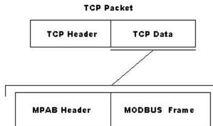
Figure 9: MODBUS TCP Frame
