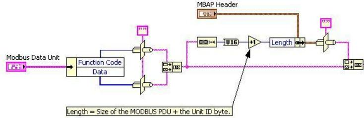
Figure 18: Format TCP MODBUS Request
