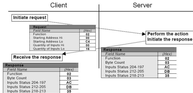
Figure 7: Complete MODBUS Transaction<sup>1</sup>
