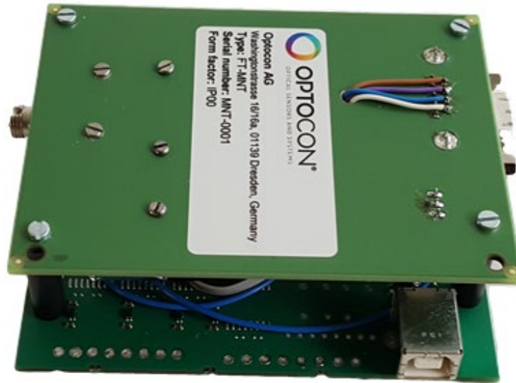
Figure 1. FOTEMP1-OEM-MNT PCB-Based Signal Conditioner/Controller.
