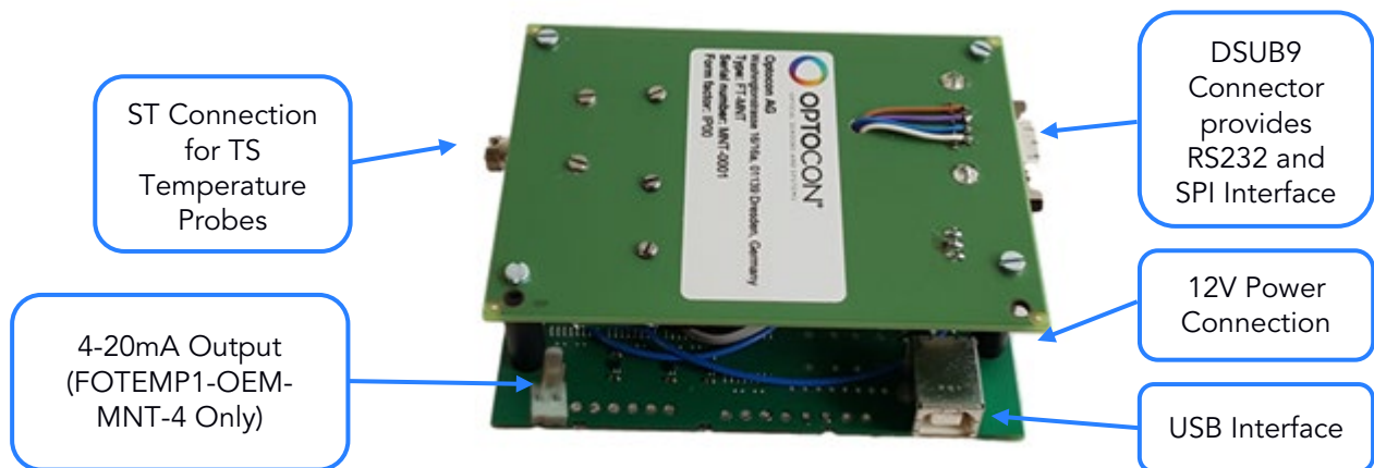
Figure 5: FOTEMP1-OEM-MNT Interface Connections
