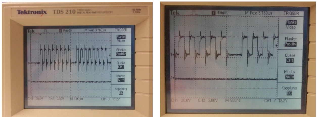
Figure 4: Oscilloscope Display Shows the "Data Gap" Between the Two Bytes
