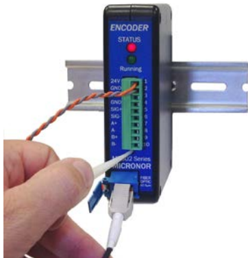
Figure 13. Location of internal CAL button for initial optical level calibration
