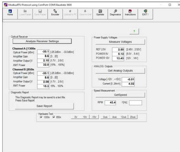
3. Click on [Operate] to view the RPM and Position Counter Value.
