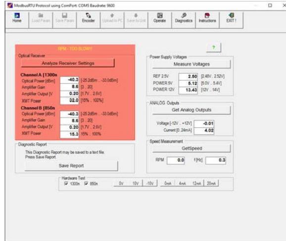
2. While rotating the shaft (RPM-Too Slow!!! Warning will go away), click on [Analyze Receiver Settings]. All measured parameters should fall within range of allowed values shown in brackets.
