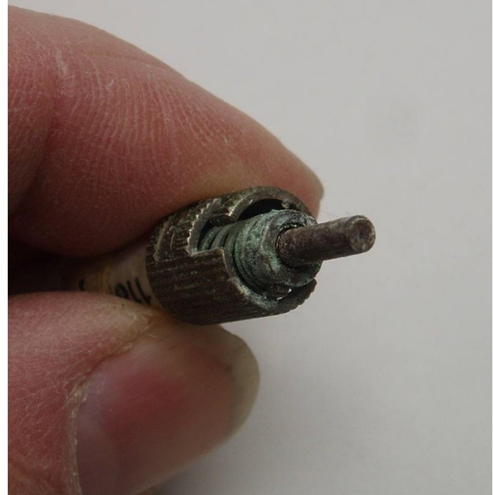
ST Fiber Connector after 1 year in operation
