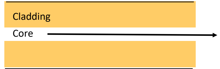
A mode travelling in a singlemode fiber
