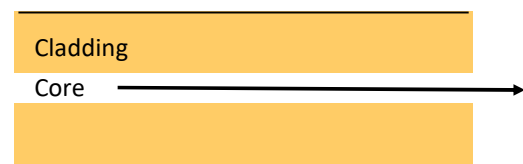
A mode travelling in a singlemode fiber
