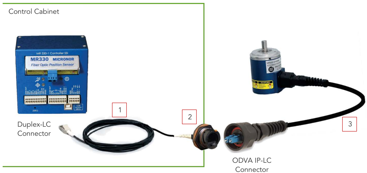
Figure 1: Typical Cabling Architecture for Harsh Environments
