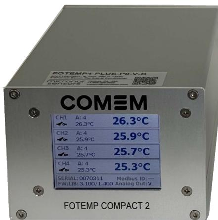
The FOTEMP C20 is designed for environments where traditional metal temperature sensors (such as RTDs, thermocouples, and capillary sensors) cannot be used, including microwave, high-frequency, high-voltage, and high-magnetic-field settings, as well as aggressive environments.
