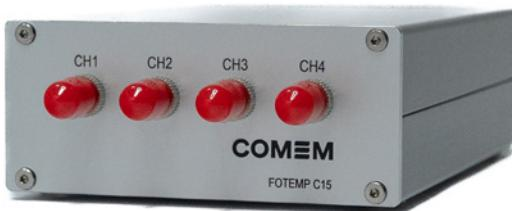
The FOTEMP C15 is designed for environments where traditional metal temperature sensors (such as RTDs, thermocouples, and capillary sensors) cannot be used, including microwave, high-frequency, high-voltage, and high-magnetic-field settings, as well as aggressive environments. It measures temperature based on changes in the optical properties of a gallium arsenide crystal (GaAs).
