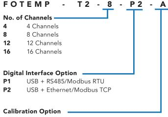
Basic, -20°C to +150°C **A1 A2** Standard, -40°C to +200°C
