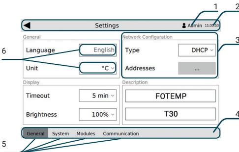
Figure 8: Sample screen with explanation of software elements
