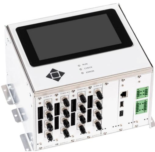
Power transformers are often vulnerable to failure during overload conditions, especially when inadequate control and protection are in place. The FOTEMP T30 is designed to measure the hot spot temperature of transformer windings in real-time.
