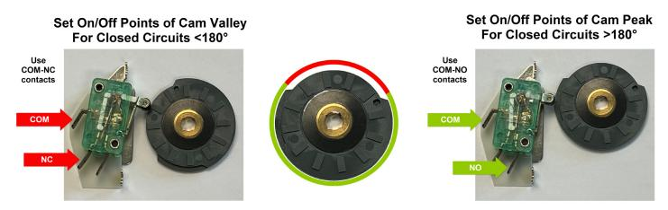
It is recommended that the user initially document his limit switch settings so it is clear whether COM/NC or COM/NO contacts are needed for a particular limit switch channel. Either a table or diagram of of the Closed/Open settings will allow the user to establish the ON and OFF points and translate them to the 0-360 scale of the internal Reference Dial and Cams.
