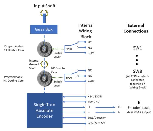
To program 4mA point, touch input Set2 to 24V DC IN and then release. The analog output will reset to 4.01mA. This should be done with the internal mechanical scale set to 360 (0) position.
