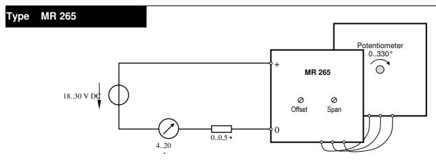
This unit produces a current ouput proportional to the setting of an externally connected potentiometer. Both the zero offset and slope of the output can independently programmed using the two on-board trimmer potentiometers.
