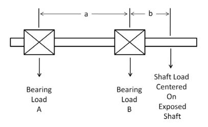
Load on Front Bearing (B) = (Shaft Load \* (a + b)) / a
