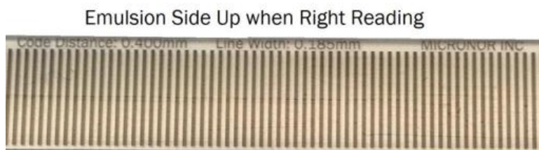
Figure 5. The emulsion side is up when right side reading text
