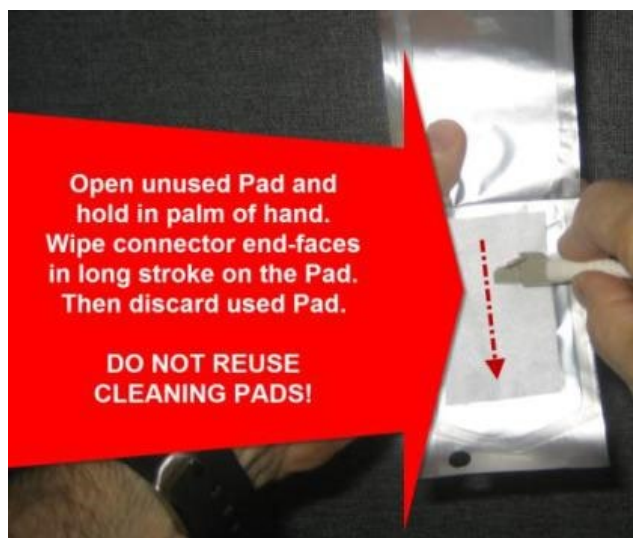
Figure 9. Clean Optical Plug with supplied Clean Wipes
