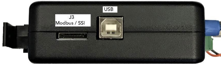
Figure 13. Location of SSI, RS485/Modbus RTU, and USB Connections
