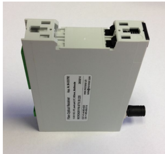
Figure 6. Close up of DIN rail adapter on module
