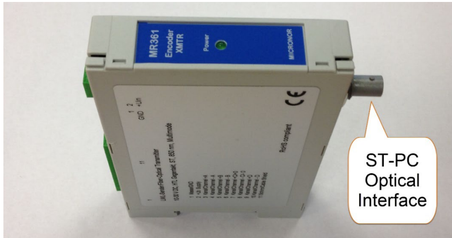
Figure 9. Location of ST optical interface on XMTR and RCVR Modules
