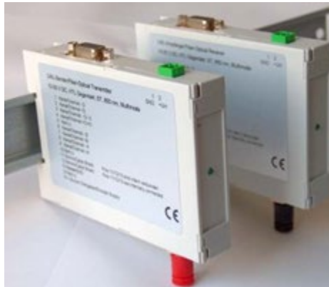
Figure 5. Modules mount on standard 35mm DIN rail
