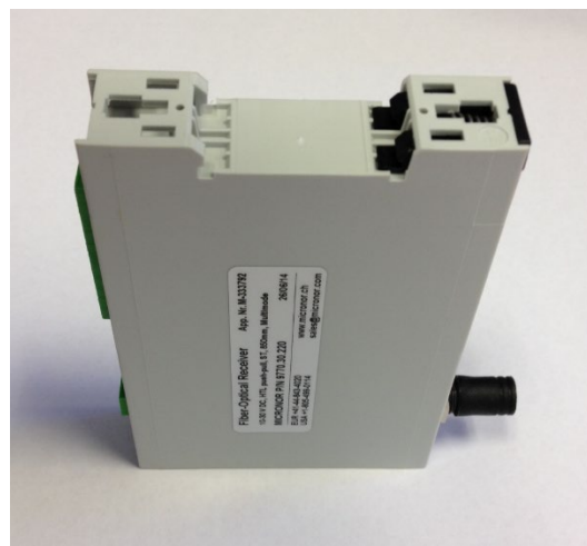
Figure 3. Close up of DIN rail adapter on module
