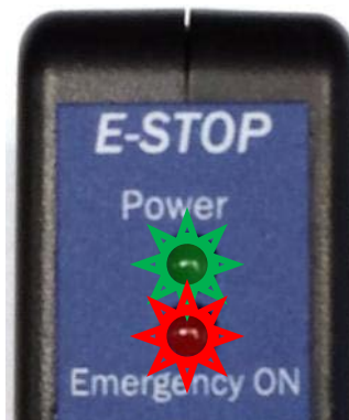
Figure 9. Properly Powered Controller with Depressed Switch, Broken Fiber Link, or High Loss
