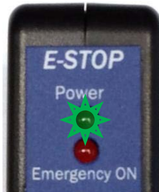
Figure 8. Properly Functioning Controller with Switch Connected and Not Depressed
