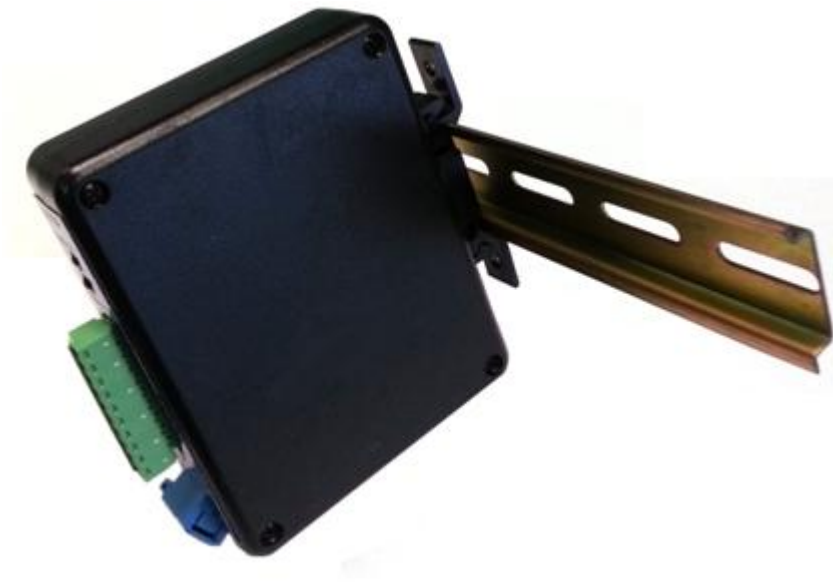
Figure 5. DIN Rail Mount
