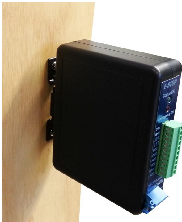
Figure 5. DIN Rail Mount
