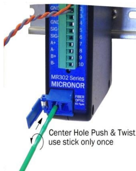
Figure 10. How to Clean Optical Interface With Cleaning Stick
