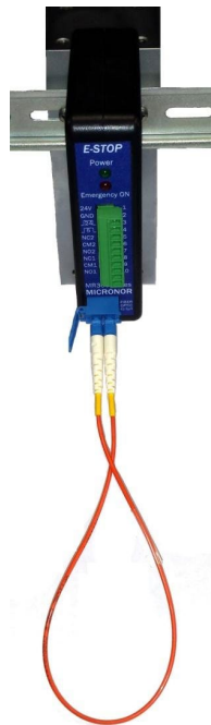
Figure 13. LC Loopback MR380-1-3 Controller Check
