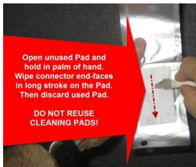
Figure 11. How to Clean Optical Plug with Cleaning Wipe
