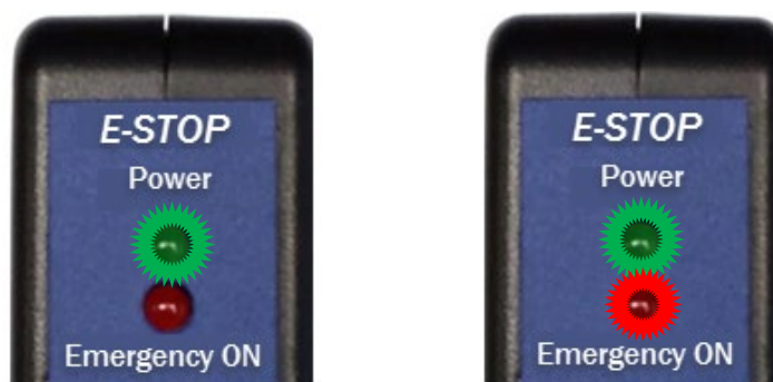
Figure 12. Controller with E-Stop: Power On (Left) and E-Stop Depressed (Right)
