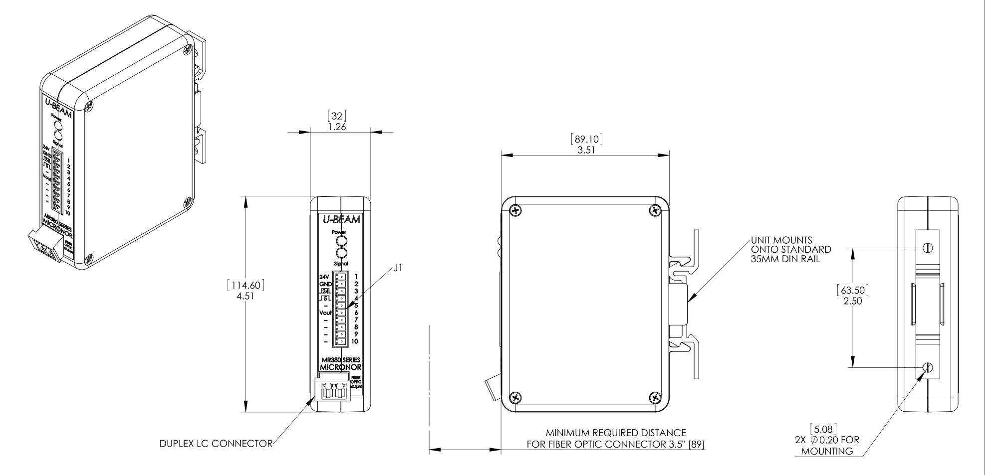
J1 PHOENIX CONTACT P/N: 1803358 (10 PIN TERMINAL), MATING PLUG P/N: 1803659
