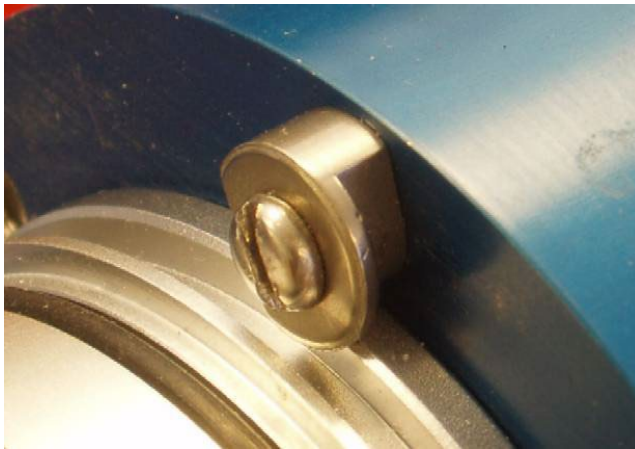
Figure 2. Sensor mounted using Servo Clamps
