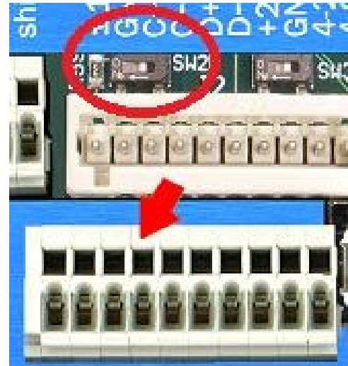
Figure 8. SSI Termination Resistor Switch
